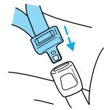
5. To put the retractor in the automatic locking mode, grasp the shoulder portion of the belt and pull downward until all of the belt is pulled out and a click is heard.
